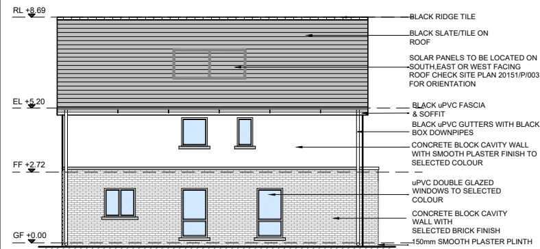
Side Elevation SCALE 1:200 @ A3 HOUSE TYPE C1
